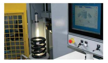
Mobile Spring Assembly Press The mobile assembly press NSP M was specially developed for bogie construction and maintenance. With it the primary spring can be efficiently and ergonomically essembled or dismantled.
