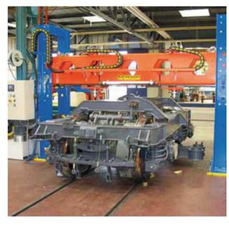
Nencki bogie presses allow bogie manufacturers and maintenance workshops uncomplicated assembly and dismantling. As a specialist in technically leading test stands, the company has valuable experience and also makes the highest demands of stability and user-friendliness for bogie presses.
